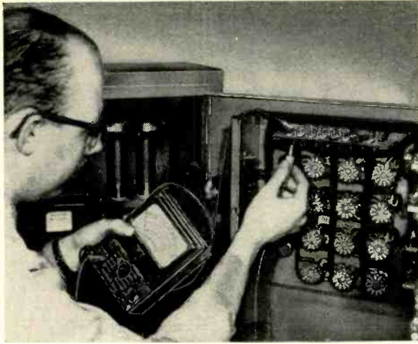
Industrial technician makes resistance checks in "brain" panel of Robotron weld timer.
